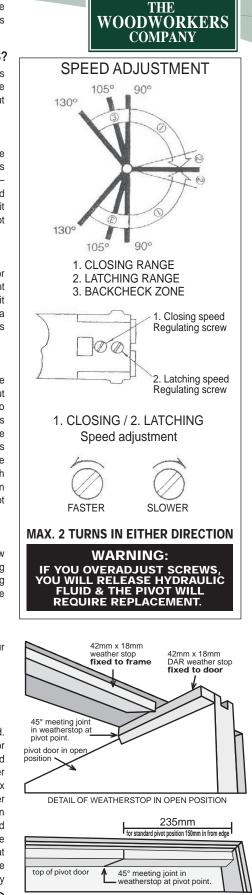
FRONT ELEVATION OF WEATHERSTOP IN CLOSED POSITION
